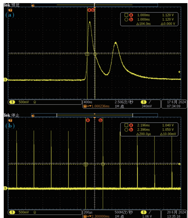
Fig.5 (a)The separately pulse Q -switched tri-wavelength laser. (b)The temporal profile of the pulse sequence
